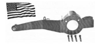
Allows 68-82 Vettes to use a 5" back spacing on an 8 1/2" to 9" wheel with a 10" or 11"" tire.
